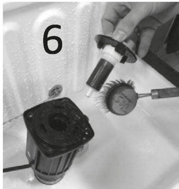
Clean rotor with water and brush
