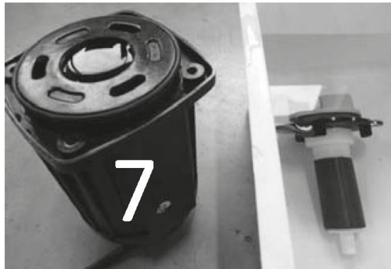
Put pump house in a vertical position and fill with a mild lime scale remover (like cleaning vinegar). Immerse rotor in a plastic bowl /container filled with the same lime scale product and leave both for 24 hours. After 24 hours rinse off with water and re-assemble pump.
